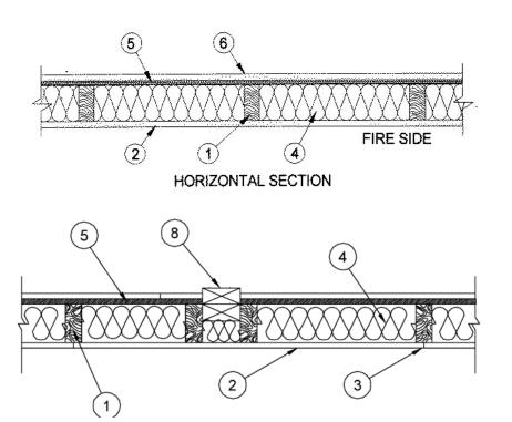
UL U356 One-Hour Fire-Resistance Rated, Limited Load Bearing Wall Assemblies for Thermo-Ply® Red & Blue Protective Sheathing Using IBC Section 722 Calculation Method
