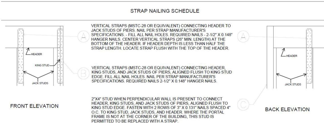
**Figure 3. Header Connection Detail - Option 1**
