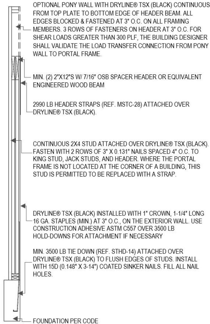
**Figure 4. PFH Option 1 Section A-A**
