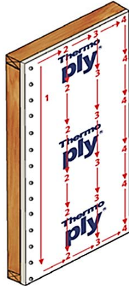
FIGURE 2. INSTALLATION INSTRUCTIONS – WRB INSTALLATION PROCEDURE
