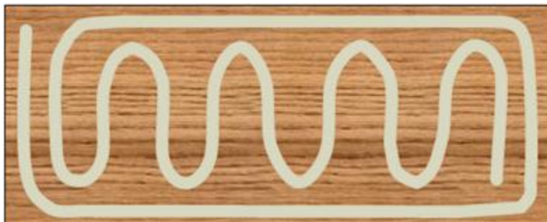
FIGURE 2. ACCEPTABLE ADHESIVE APPLICATION PATTERN
