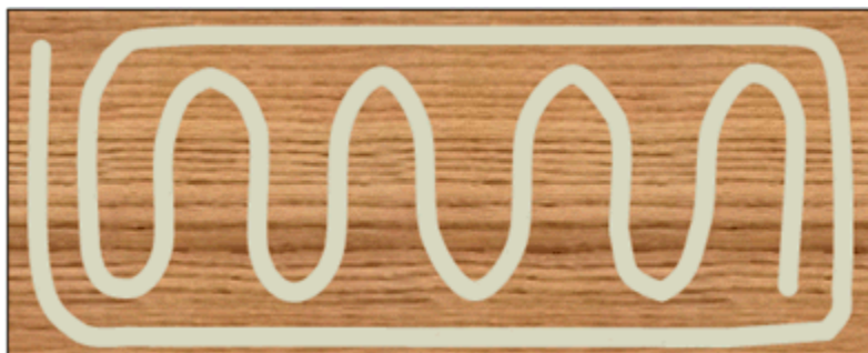
FIGURE 2. ACCEPTABLE ADHESIVE APPLICATION PATTERN
