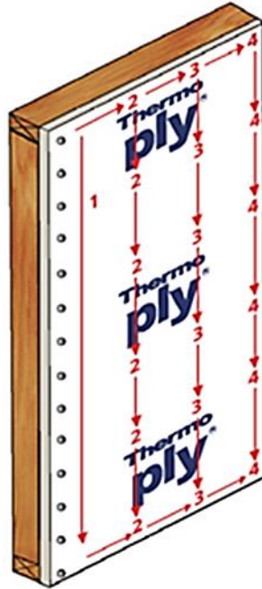
FIGURE 2. INSTALLATION INSTRUCTIONS – WRB INSTALLATION PROCEDURE
