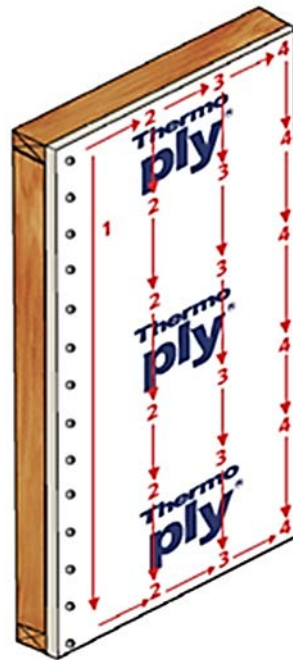
FIGURE 2. INSTALLATION INSTRUCTIONS – WRB INSTALLATION PROCEDURE
