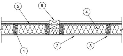
UL U356 One-Hour Fire-Resistance Rated, Limited Load Bearing Wall Assemblies for Thermo-Ply® Red & Blue Protective Sheathing Using IBC Section 722 Calculation Method
