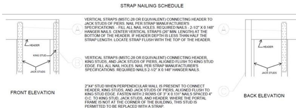
Figure 3. Header Connection Detail – Option 1
