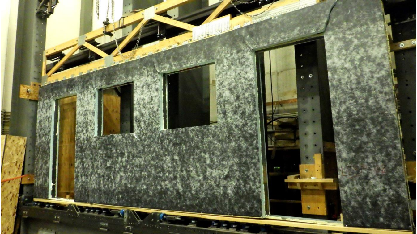
Figure 1. H-SIS-SAG Assembly with Interior GWB – Wall Application
