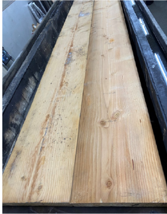
Figure 2. Lumber Treated with MFB-34 CitroTech
