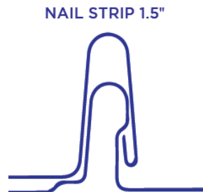
Figure 7. Compatible Panel Seams – PV Cube KLOC
