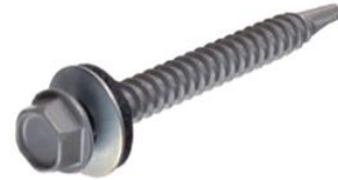
#14 x 1 1/2" T-5 Self-drilling, Fenderhead Dyna-Coat Coated HWH Screw with EPDM Washer
