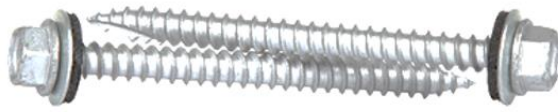
#14 x 2" Self-tapping Type-17, Type A, Dyna-Coat Coated HWH Screw with EPDM Washer
