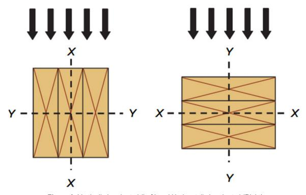
Figure 3. Vertically Laminated (Left) and Horizontally Laminated (Right)
