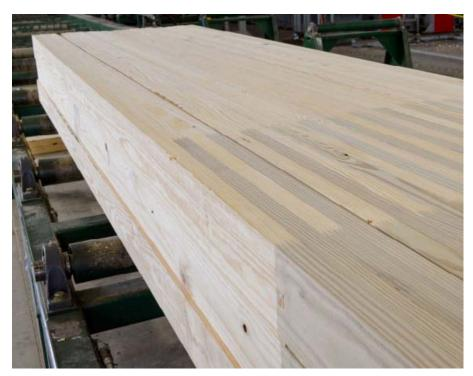
Figure 2. Staggered Laminations
