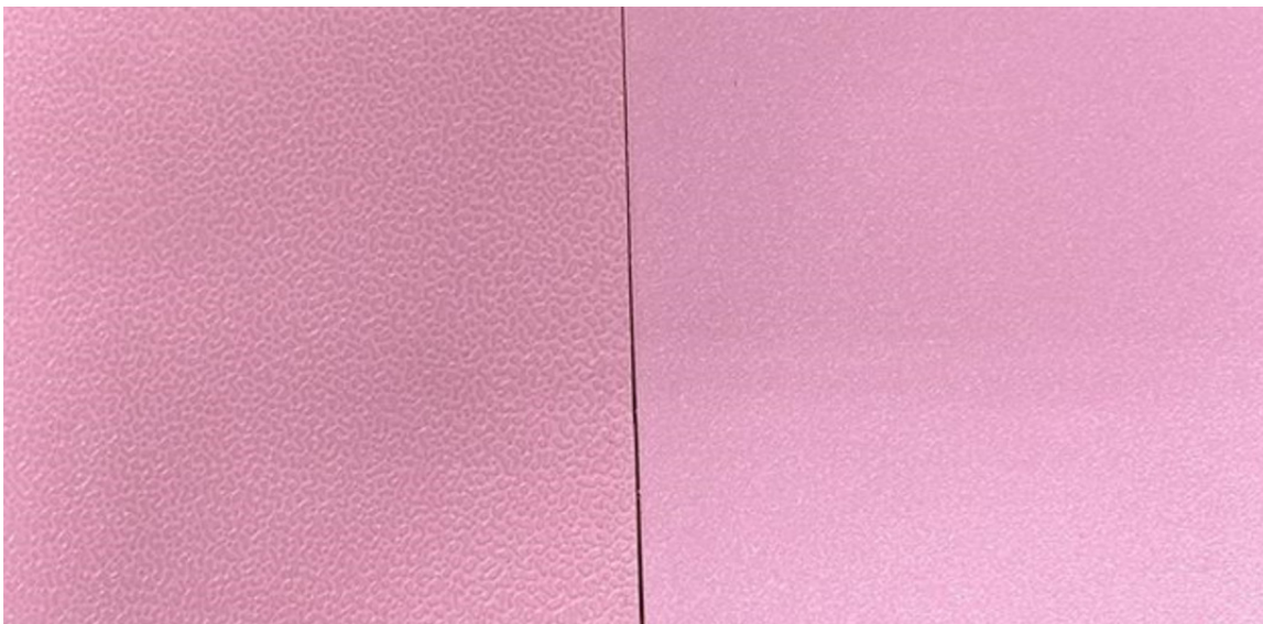
Figure 3. OC SIS Panel Facers – Haircell (Left) and Medium Matte (Right)
