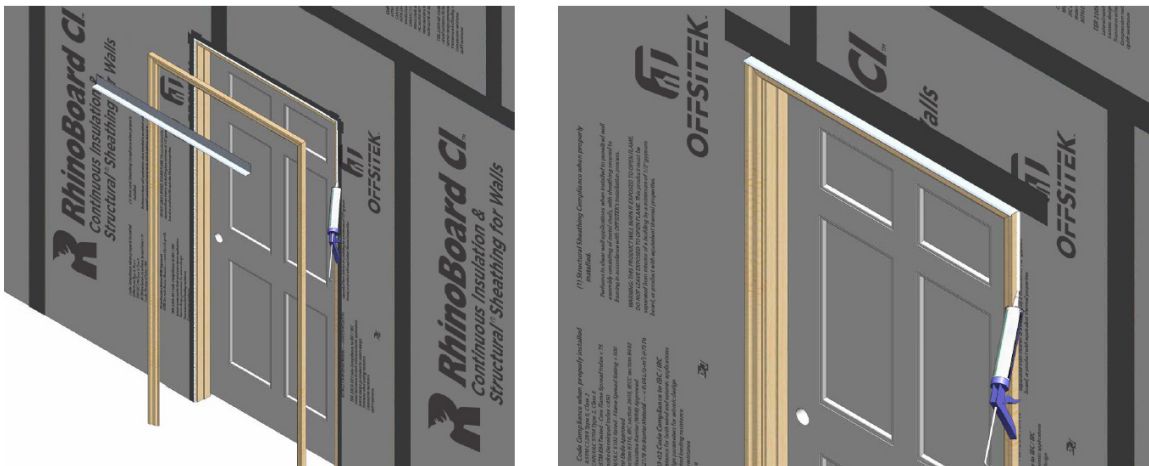
Figure 9. Seam Tape Installation Details – Door Finishing Details
