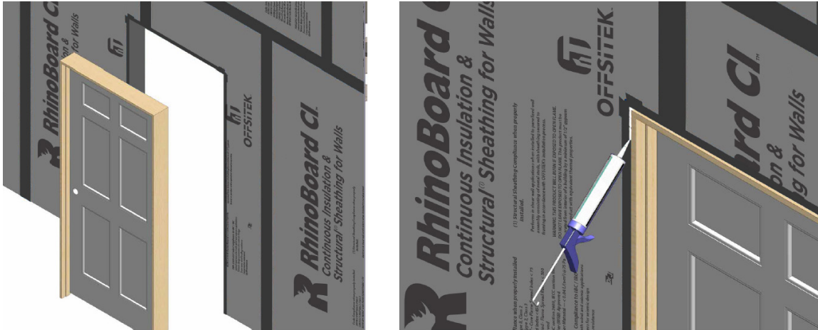
Figure 8. Seam Tape Installation Details – Doors
