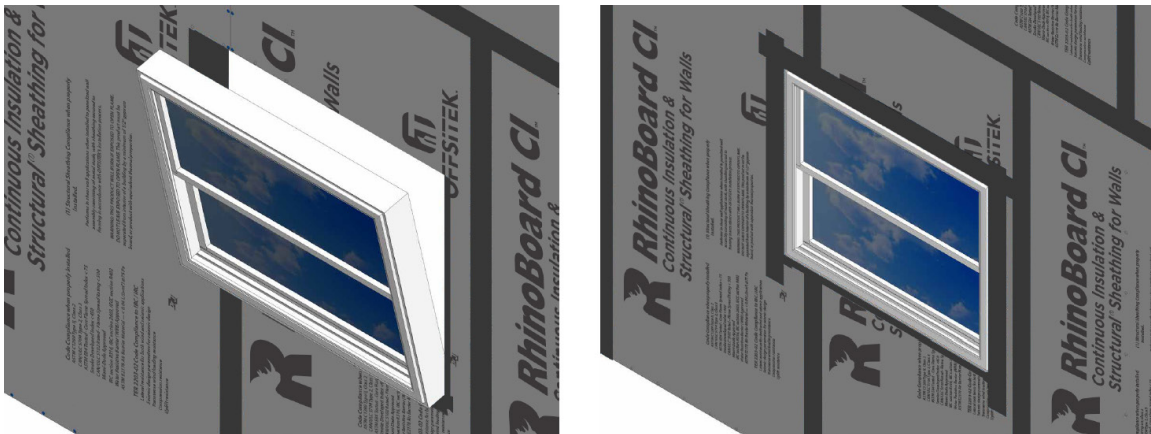
Figure 7. Seam Tape Installation Details – Windows
