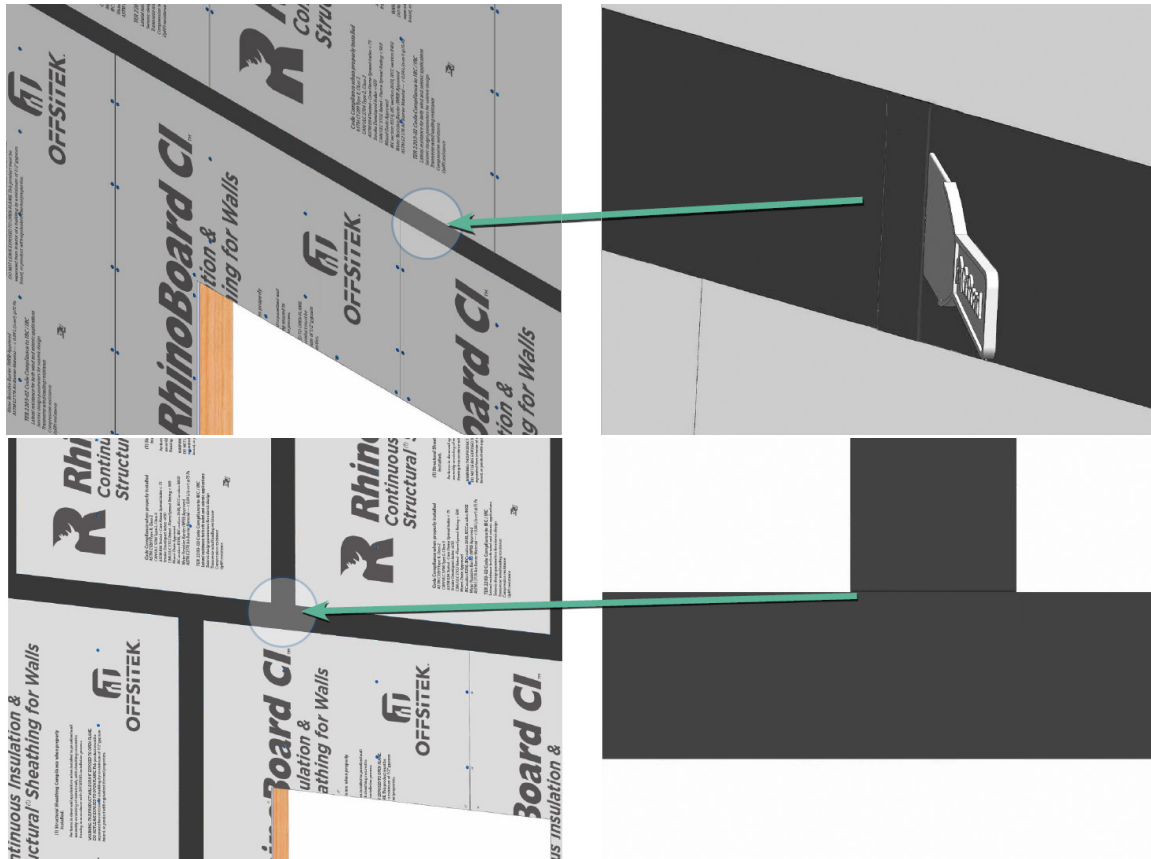
Figure 5. Seam Tape Installation Details
