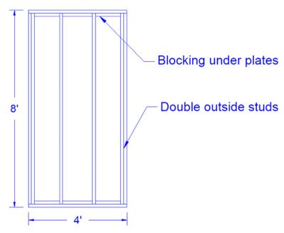
Figure 3. Framing Configuration 2
