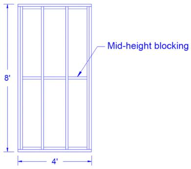
Figure 4. Framing Configuration 3
