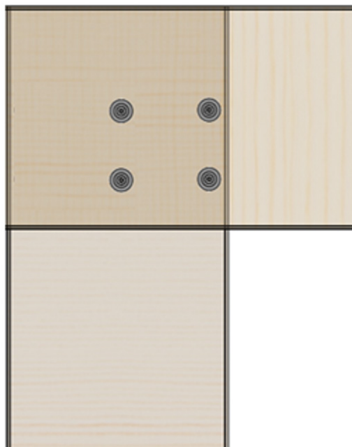
Figure 6. Beam over Notched End Post using CAMO Series \frac{5}{16} " PROTECH Ultra 4 Coated Flat Head Screws
