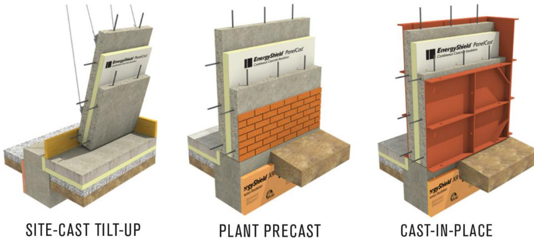
Figure 1. Applications EnergyShield PanelCast TriLam
