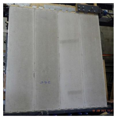
Figure 1. C-SIP Used in the CSP Insulated Interlocking Plug-N-Play Panel System
