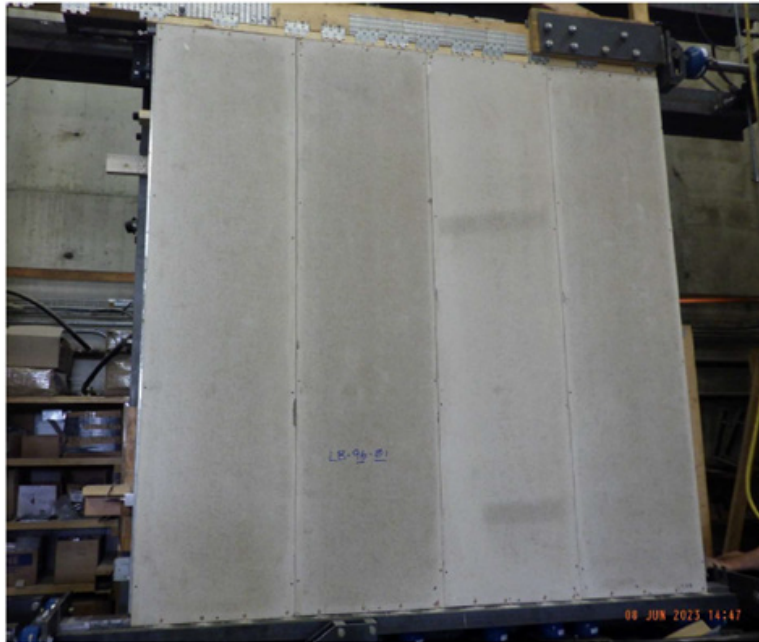
Figure 1. C-SIPs Used in the CSP Insulated Interlocking Plug-N-Play Panel System
