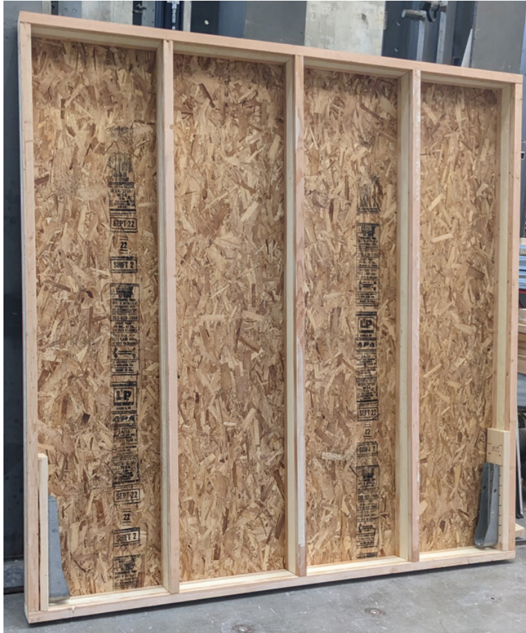
Figure 2. Insul-Stud Structural Insulated Stud Wall Assembly
