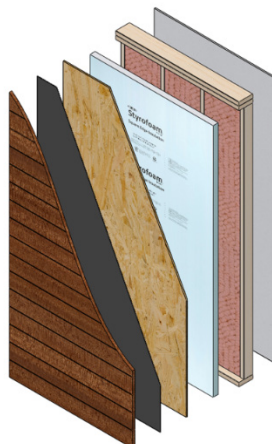
Figure 1. DuPont Styrofoam Extended Plate Wall System
