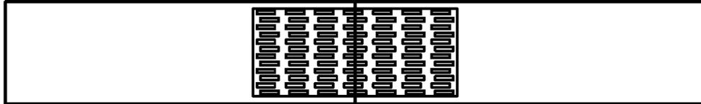
Standard test joint for steel tension parallel to slots
