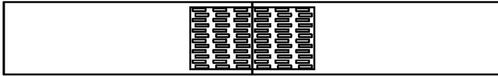
Non-standard test joint for steel tension parallel to slots
