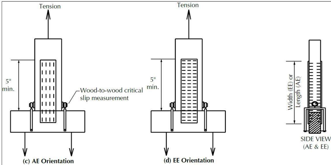
**Figure 3.** AE and EE Orientations (From TPI 1 Figure 5.2-3)
