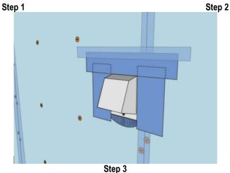
Figure 2. Typical Penetration Flashing Detail - Flanged
