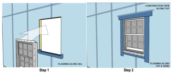
Figure 4. Typical Window Flashing Detail
