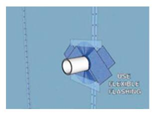
Figure 3. Typical Penetration Flashing Detail - Unflanged
