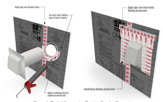
Figure 2. Typical Penetration Flashing Detail - Flanged
