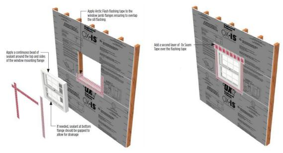
Figure 4. Typical Window Flashing Detail
