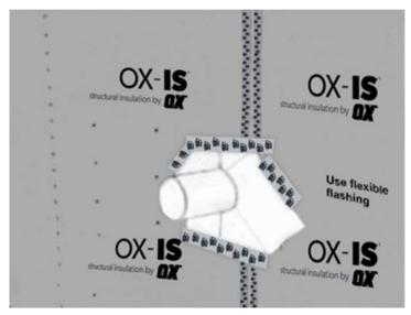
Figure 3. Typical Penetration Flashing Detail - Unflanged
