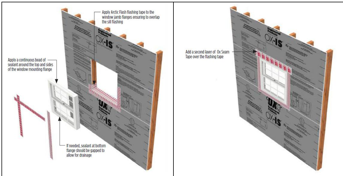
Figure 6. Typical Window Flashing Detail
