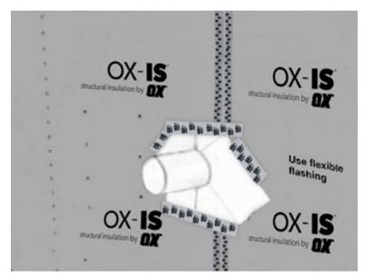
Figure 5. Typical Penetration Flashing Detail – Unflanged
