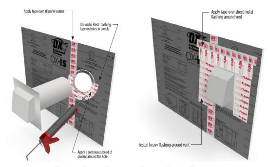
Figure 4. Typical Penetration Flashing Detail - Flanged
