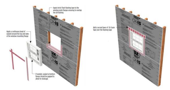
Figure 6. Typical Window Flashing Detail
