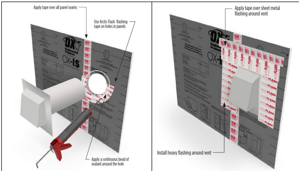
**Figure 4. Typical Penetration Flashing Detail – Flanged**
