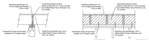
Figure 4. Section Views of FrameFAST Fasteners with Blocking
