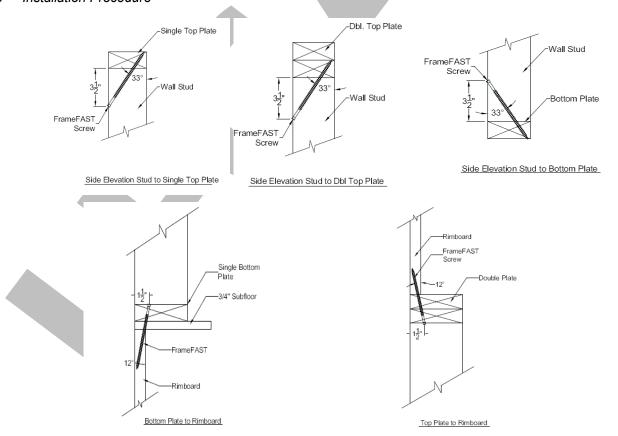
Figure 3. Installation of FrameFAST Fasteners for Specific Applications
