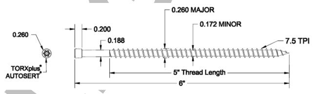
Figure 1. FrameFAST Fasteners Specification
