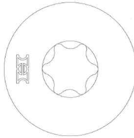
Figure 3. ConnexTite Fasteners Countersunk Head Detail
