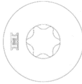
Figure 3. ConnexTite Fasteners Countersink Head Detail
