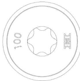
Figure 1. ConnexTite Fasteners Flange Head Detail
