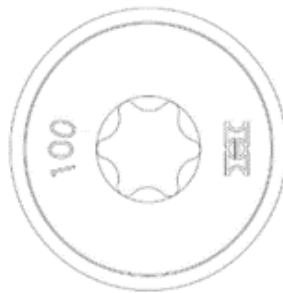
Figure 1. ConnexTite Fasteners Flange Head Detail
