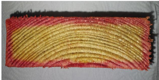
Figure 1. Dye reaction method shows chemical penetration in wood substrate. Red color indicates borate penetration following AWWA A3-05 Standard Methods for Determining Penetration of Preservatives and Fire Retardants.
