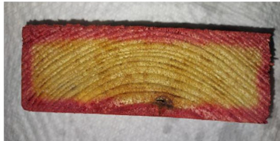
Figure 1. Dye reaction method shows chemical penetration in wood substrate. Red color indicates borate penetration following AWWA A3-05 Standard Methods for Determining Penetration of Preservatives and Fire Retardants.
