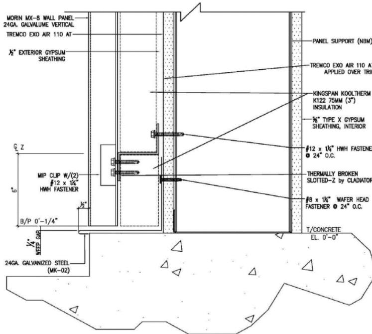
Figure 7. Typical Base Detail
