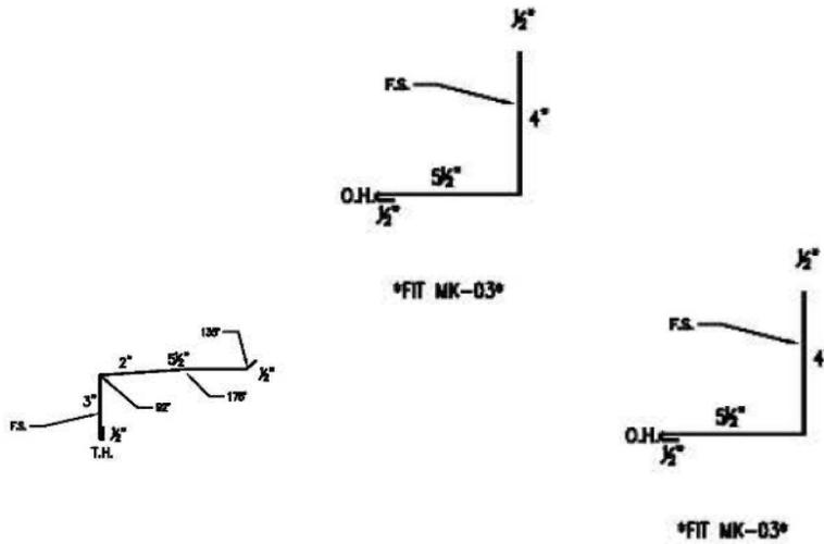
Figure 8. Flashing Profiles
