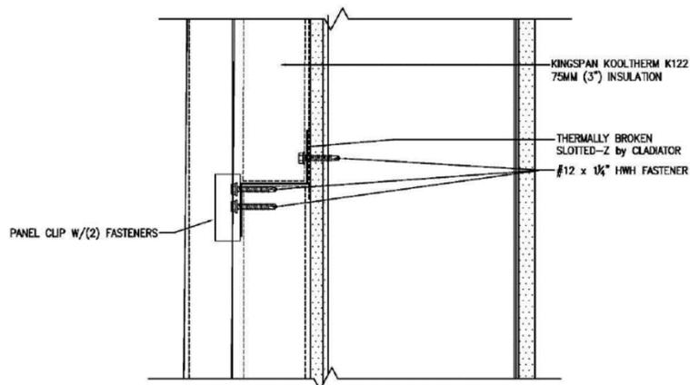
Figure 4. Typical Slotted-Z Detail
