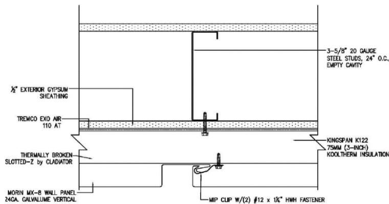
**Figure 6.** Typical Vertical Panel Joint Detail
