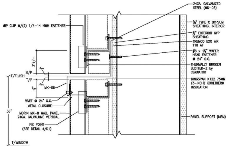
**Figure 5.** Typical Stack Joint Detail
