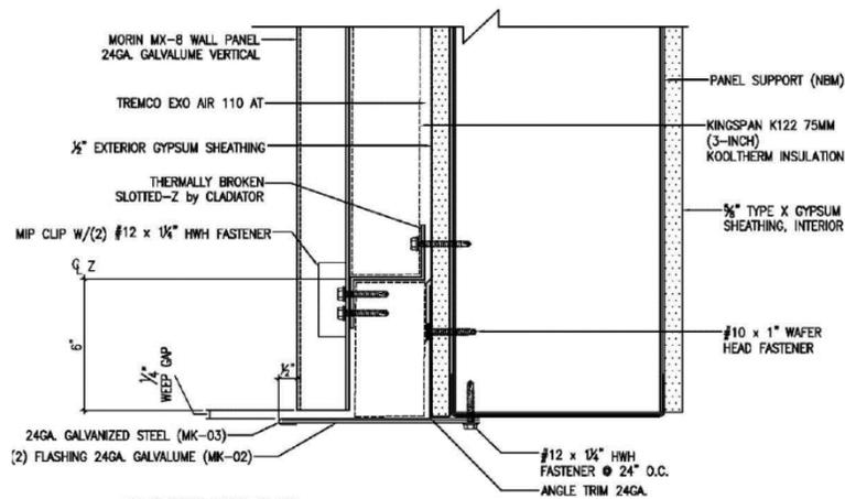
Figure 3. Typical Window Head Detail
