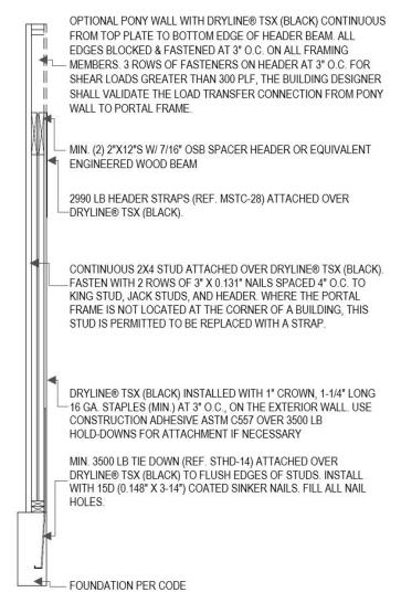
Figure 4. PFH Option 1 Section A-A
