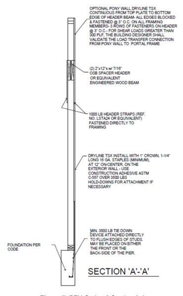
Figure 7. PFH Option 2 Section A-A
