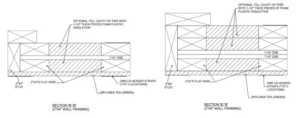
Figure 5. PFH Option 1 Section B-B
