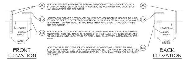
Figure 6. Construction Details of DRYline® TSX (Green) 12" to 24" PFH - Option 2
