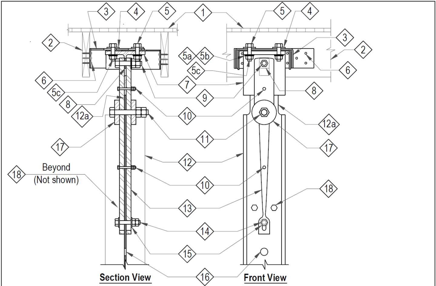
**Detail of SkinnyBrace and Connections to Floor Framing**
