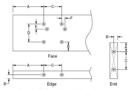
Figure 3. FlatLOK Fasteners Edge and End Distance Requirements
