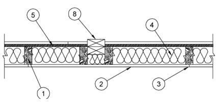
UL U356 One-Hour Fire-Resistance Rated, Limited Load Bearing Wall Assemblies for Thermo-Ply® Red & Blue Protective Sheathing Using IBC Section 722 Calculation Method
